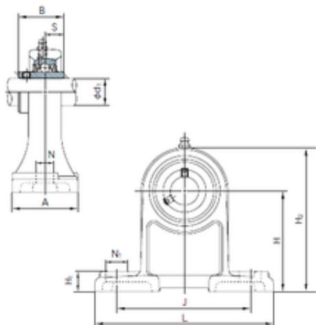
UCPH205 Bearing 2D drawings and 3D CAD models
